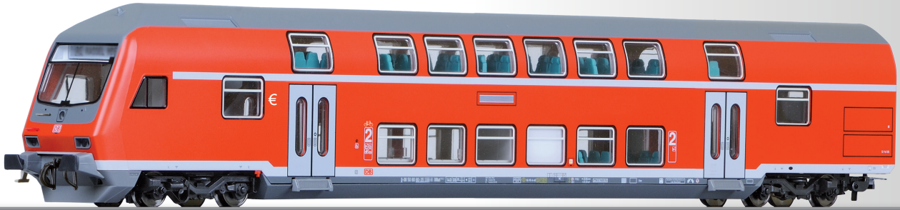
Doppelstock-Steuerwagen 2. Klasse DBbzf 761 der DB AG 2nd class double-deck driving cab coach DBbzf 761 of the DB AG
